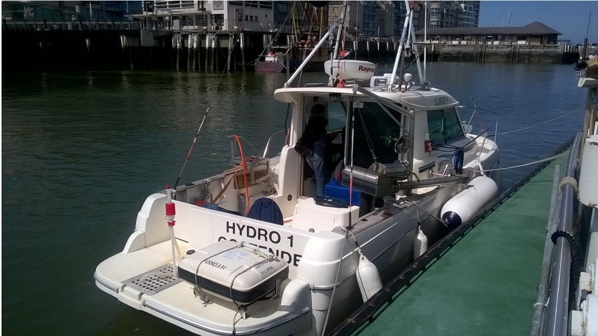
Survey vessel Hydro 1(Flemish Hydrography). The echosounder pole and orange cable are seen on the left (port side). On starboard side the pole-mounted Octans motion sensor and multibeam unit can be seen.
